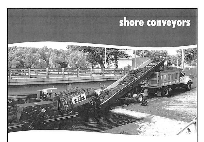
Shore Conveyors are deployed at the waters edge and serve the harvesters, transport barges and trash skimmers as an unloading link between land and water.
