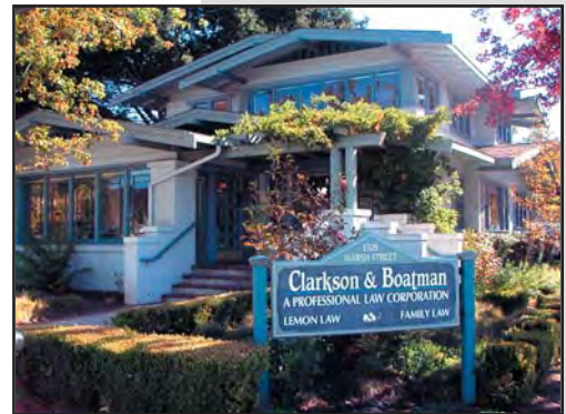
VARIATION IN ROOF AND WALL PLANES HELP BREAK UP THE FRONT FACADE.
