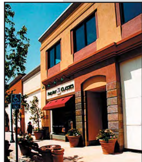
USE OF COLOR, ARRANGEMENT OF FACADE ELEMENTS, AND CHANGES IN MATERIALS HELP TO ARTICULATE THIS BUILDING FACADE
