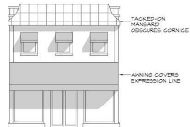
B – Improper Treatments
