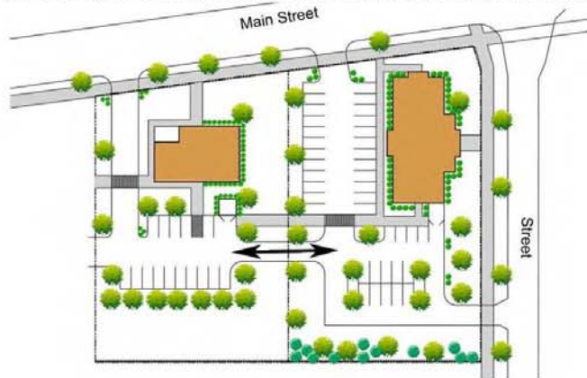
Figure 26 Illustration of Inter-parcel Access Requirements
