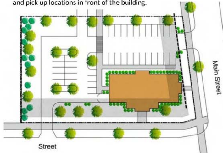
Figure 25 Parking Orientation to the Rear and Side
