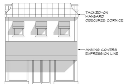
B – Improper Treatments
