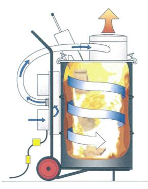
Fueled with wood or charcoal, the ELASTEC Drug Terminator's high velocity blowers create a cyclone of intense heat. A whirlwind of combustion reduces the burned material into a tiny pile of sterile ash with minimal air emissions.
