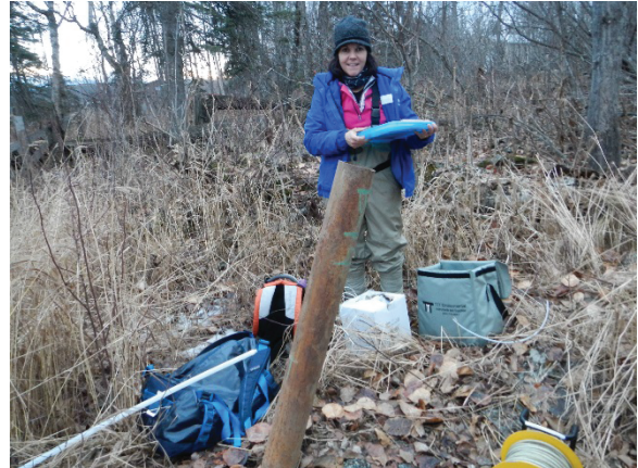
Photo 2: MW14 pulled over at 30° angle
