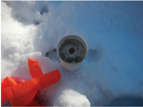
Photo 1: Ice frozen to top of casing, MW6
