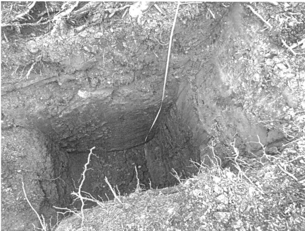
Typical soil profile for test pits; fill over peat over silt
