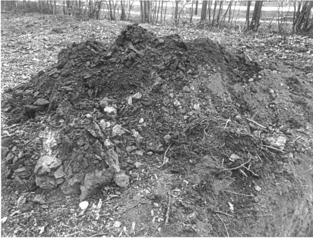
Typical soil on the parking expansion site: silt on bottom left, peat on top, fill material on bottom right
