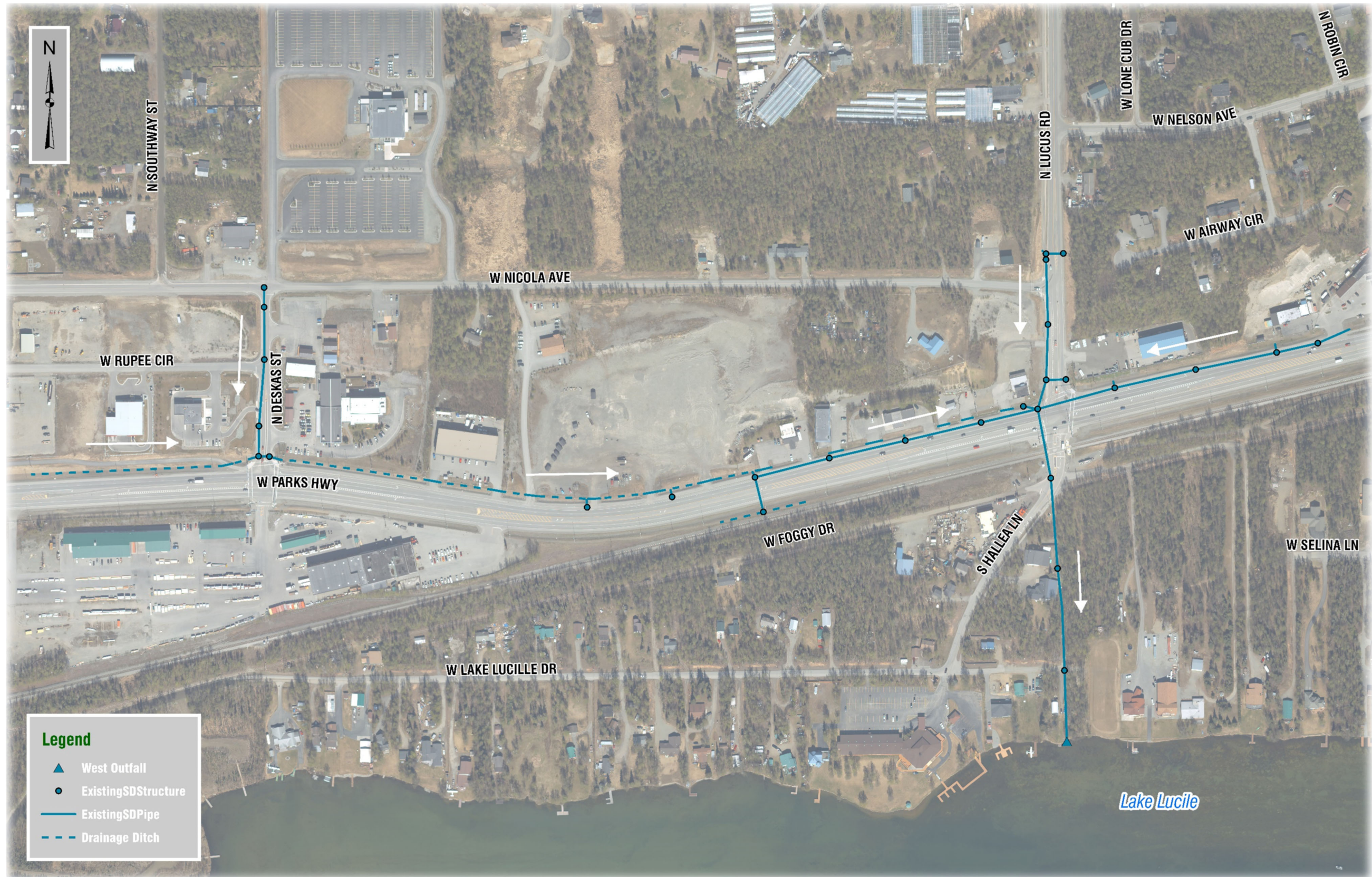
Figure 3: Drainage Patterns in the West Drainage Area
