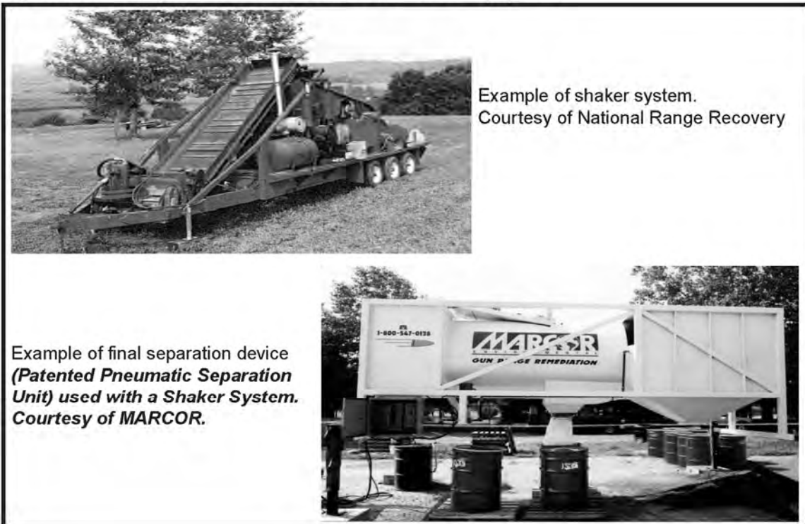
Figure 3-3 – Examples of Common Lead Reclamation Equipment
